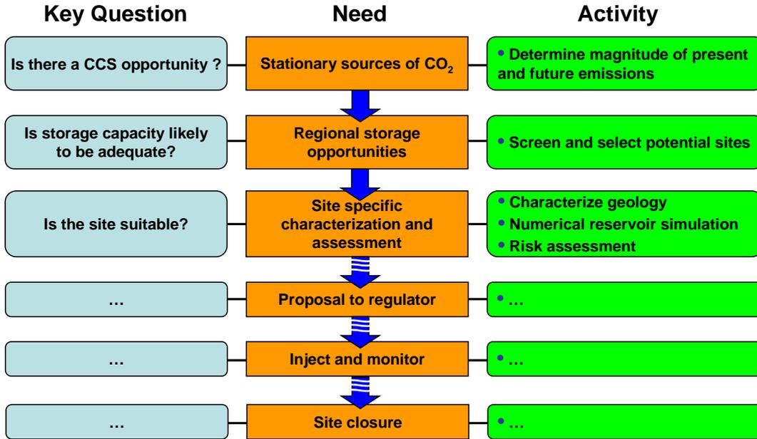
**Figure 3:** Life cycle of a CO<sub>2</sub> storage project (modified after IPCC (2005)).
