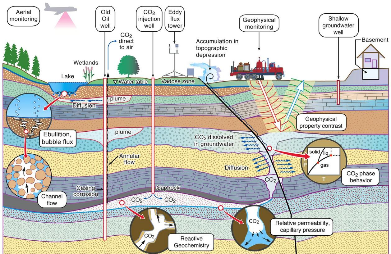
**Figure 2:** Principal processes, leakage risks, and monitoring techniques associated with CO<sub>2</sub> storage in geological formations (Figure courtesy of Lawrence Berkeley National Laboratory).
